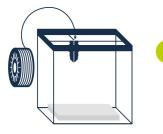
Place *P-filament Carbon 411* into your 3D printer. For complex geometries you have to use *P-support 279*. It is not required to dry both filaments prior to use.
