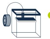
Heat up the extruder temperture to **230°C**, recalibrate your printing platform and start printing. To remove the finished part without destruction, the printer bed has to be heated to about **110°C**.
