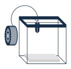
1 Place *P-fila* rept 721 into your 3D printer. For complex geometries you have to use *P-support 279*. It is not required to dry both filaments prior to use.
